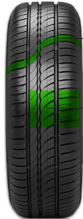
DIZAJN GAZNOG SLOJA SA SPECIFIČNOM SEKVENCOM DEBLJINE: NISKA RAZINA BUKE U VOZILU
