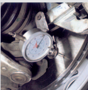
► Measuring disc run-out on the vehicle
