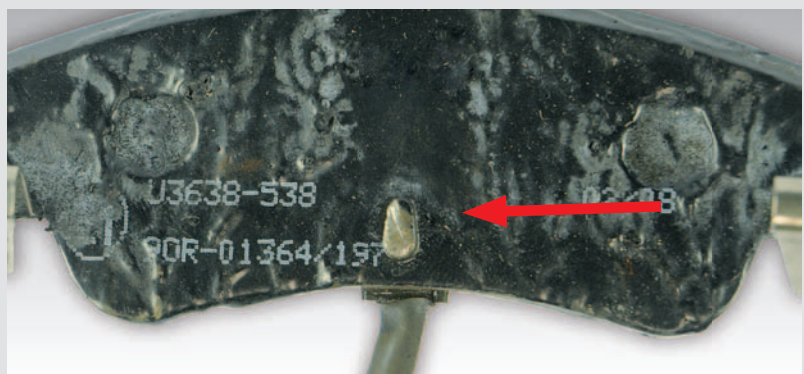
► Piston imprint on the positioning device
