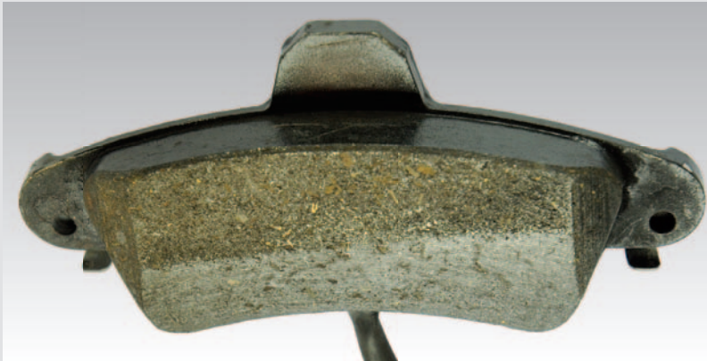
► Pad with inadequate contact pattern
