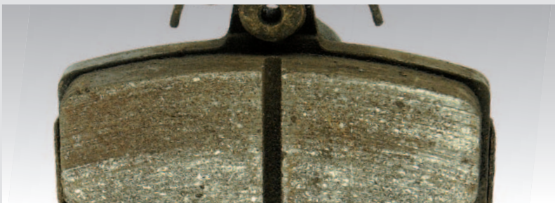
► Contamination of the friction surface
