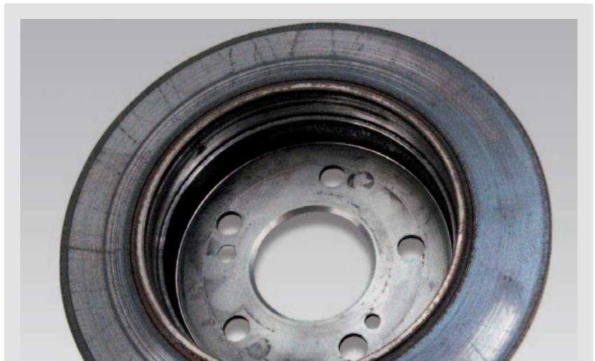
► Brake disc with static spots
