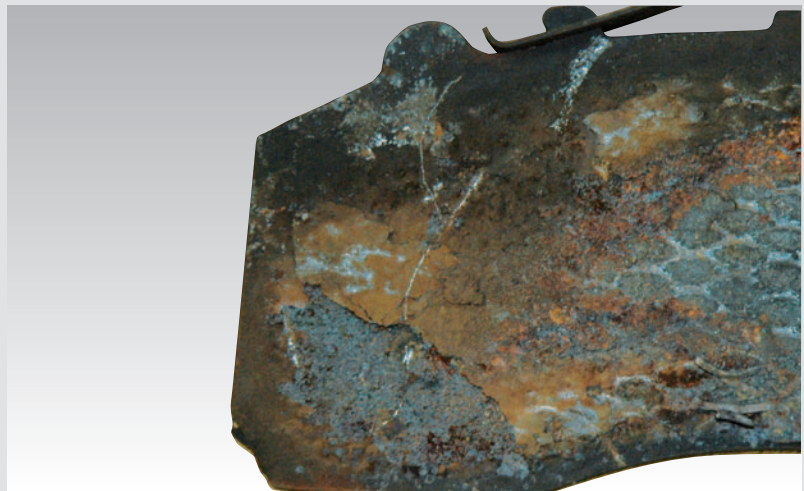
► Heavy underlying corrosion
