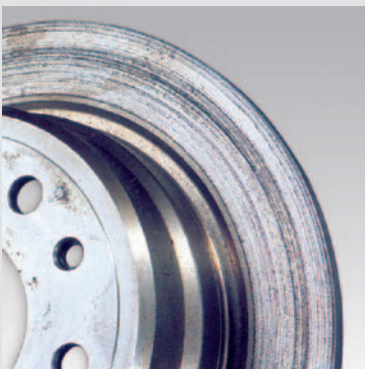
► Brake discs damaged by worn friction material
