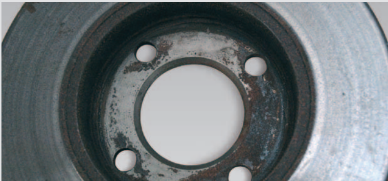
▶ Heavy underlying corrosion
