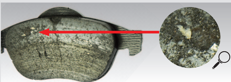
► Residues – metal pick-ups in the pad surface
